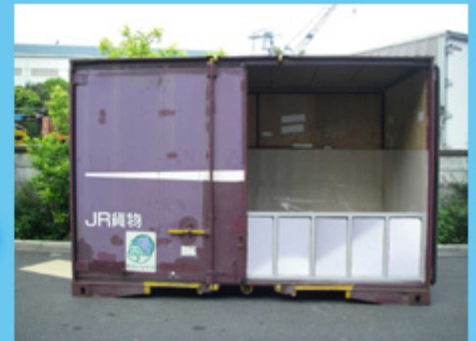
2 layers PE(0.3mm per layer)
